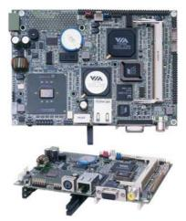
The HS-2606 is a 100/133MHz FSB VIA CLE266/VT8235 chipset-based board designed for Mini PCI Local Bus ULV Intel® Celeron® processor 400/650MHz. These features combine and make the HS-2606 and ideal all-in-one industrial single board computer. Additional features include and enhanced I/O with CF, PCMCIA, CRT/Panel, audio, LAN TV-Out, 4 COM, and USB2.0 interfaces.
